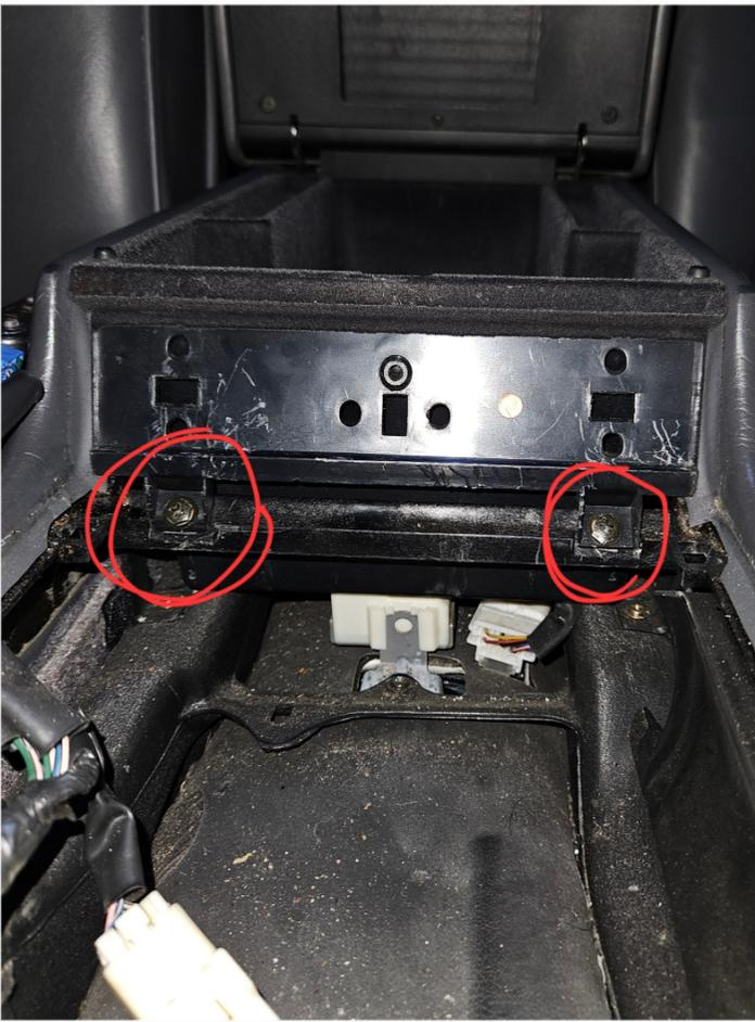
This part where you remove the console box is kinda of tricky due to the shape of it as it has this type of hook shape that can't be seen until fully taken out. But what you want to do is try and lift the console box up from the front, though when doing that it'll stop moving as it gets stuck on the plastic piece that held the screws in for it. So you want to gently force it from under to go up. If done right ill come out with no issue
