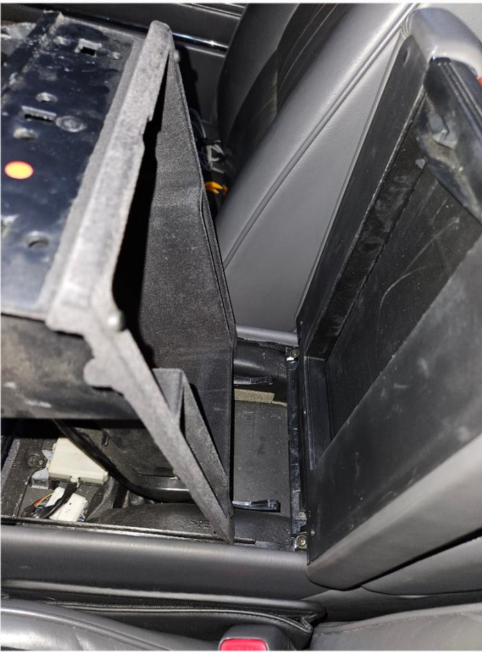
You want to lift it up like that in the photo and gently pull and wiggle it out to remove the console box.
