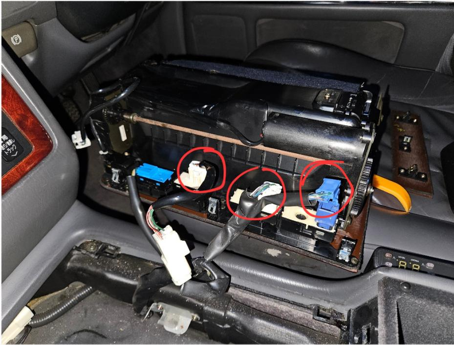
What i did for this since one of the blue connectors is hard to unplug is that I moved my driver seat all the way up, then unplugged the connectors i circled in red then layer to top of it flat on the seat for now.
