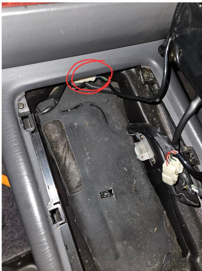
The circled spot is the connector that's held down by a clip. Unplug that one first.
