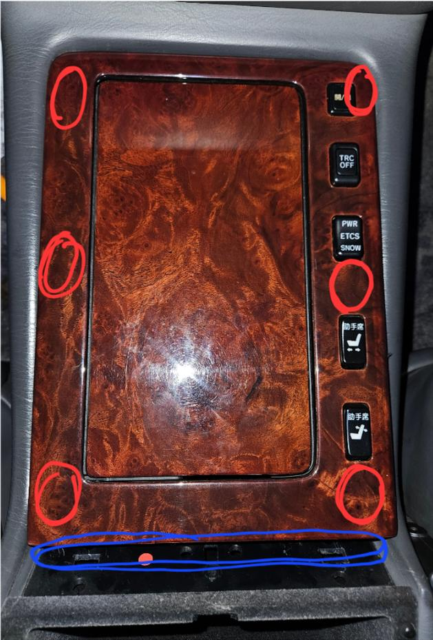
In the red are where the 6 clips are. Also watch out for the connectors on the right when prying. But I'd recommend to start prying where I circled in blue.
